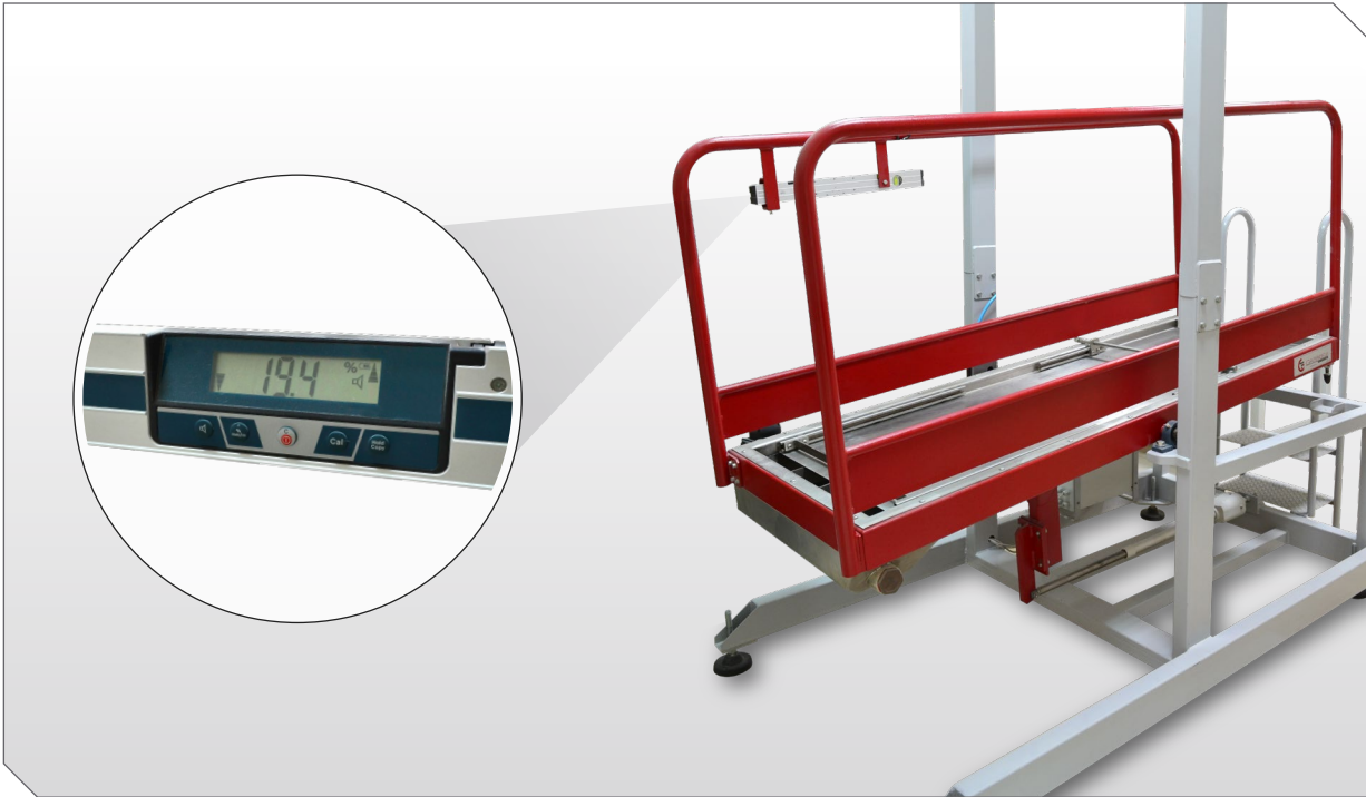
Ramp used to test anti-slippery properties
