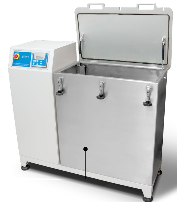
Apparatus used for laboratory testing of frost resistance of ceramic tiles.
