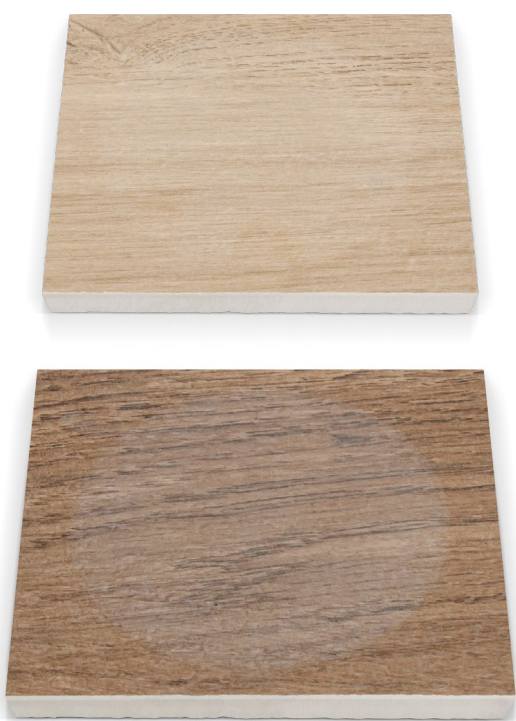
Comparison of two tile fragments after the surface abrasion test (number of rotations – 2100)
